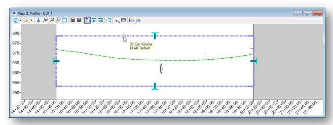
When the element is selected, four handles appear that allow adjusting the extents of the bounding area, as shown above.
