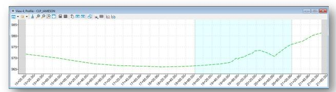
**Note:** The profile is displayed in the profile view for review and editing; however, the profile is not written to the design file. The selected view window is used as a temporary display of all the profiles associated with the selected alignment. The selected view window is not specifically associated with an alignment/profile and can be used to display the profiles from different geometric alignments as needed.
