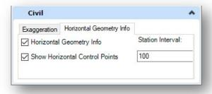
The **Horizontal Geometry Info** option toggles on the display of the geometry tangent length, and length and radius for horizontal curves. This information is displayed across the top of the profile window as shown below.
