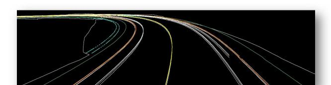
Only the top template points are used to create the proposed surface mesh. Points below the surface are excluded from the proposed design surface.
