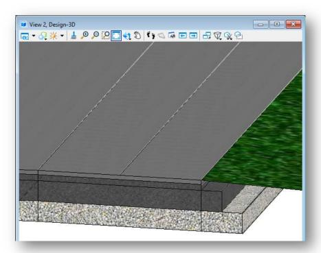
When the template is processed, the template points are connected between template "drop" locations to form the longitudinal break lines that are used to create the proposed surface. An example of the longitudinal break lines plotted from a 3-dimensional design surface is shown below.
