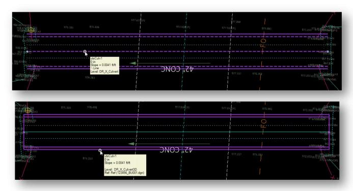
The Subsurface Utility software also creates a 3D model in the drainage basemap named "Design-3D" containing the 3D model of the box culvert as shown below.
