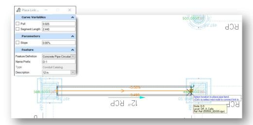
A line is placed in the current 3D model that can be used to modify the link. The extruded 3D link is placed in the 3D model as shown below.
