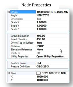
Currently the Node invert elevation will automatically change to match the lowest connected conduit invert elevation. Until this behavior is addressed by the software it is best practice to set all pipe begin and end invert elevations then set the node invert.
