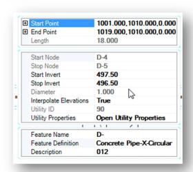
From the *Properties* menu, shown at left, the **Start Invert** and **Stop Invert** values can be edited if necessary to set the correct elevations for the pipe.
