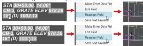
• The (D) standards for direction and must be manually typed in. This is the direction the pipe is going away from the node.
