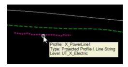
**Note:** The Utility feature definitions are set up to project the top of the conduit (not the invert) whereas Sanitary and Drainage project the bottom (invert).
