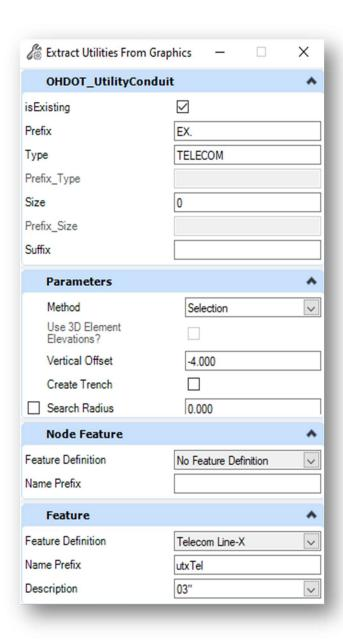
When the **Method** parameter is set to **Selection**, the dialog inputs are as follows:
