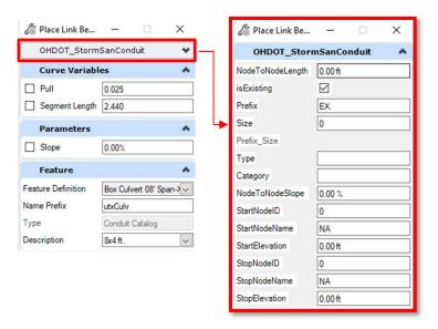
Feature definitions for existing and proposed box culverts are provided in the ODOT standards. The available features for existing box culverts are shown on the following page. The span and rise for each available culvert feature is defined by the **Description** field as shown at right above.
