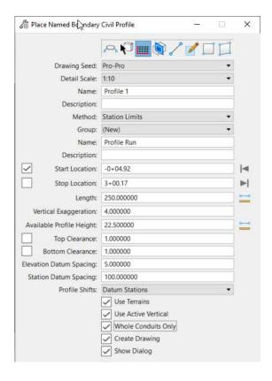
In the create Drawing dialog that opens make sure to set the drawing model scale to match the scale set in the place named boundary dialog.
