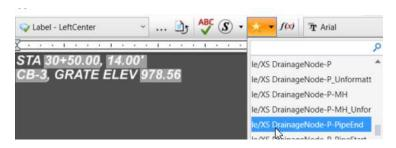
• After selecting the text favorite, it will be inserted into the text editor dialog. But the fields within the text favorite still need to be assigned to an element to know the property values to display. To do this you simply right click on the field and select reassign then select the element to assign the field to. Repeat this for all the fields.
