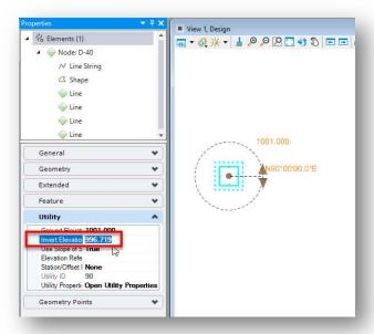
**Note**: The Filters are set up to search within a 12foot buffer of the cell. There is a chance that the process could not find the FLINE cell or find and use the wrong FLINE cell. Each structure should be verified the correct invert elevation is set.
