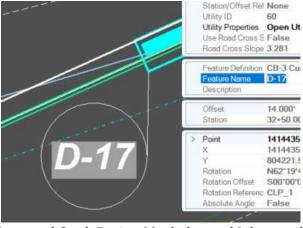
Note: Element annotation has been defined for Proposed Catch Basins, Manholes, and Inlets to place these call outs.
