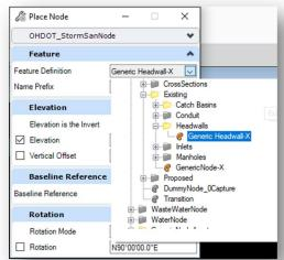
Place a node at each end of the box culvert using the **Generic Headwall-X** feature definition as shown above.
