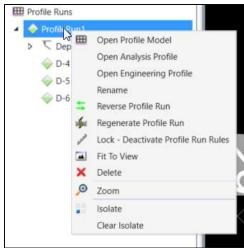
There are several options in the right click menu of a profile run, as shown above. The profile run will also have linear element in the 2d plan view to represent the profile run. If using the ProfileRun1-4 feature definitions, then the 3d plan view graphic will be on the SC\_ProfileRun1-4 level(s). note that the priority on these levels is set to be under the DR\_P\_Storm\_Sewer level so it might be covered up by that level.
