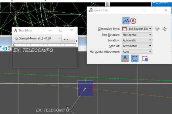
• If the <u>Alternative workflow for projecting utilities</u> section was used to show utility profiles on centerline profile, then annotation can be dynamically pulled from the utility properties using text favorites with the **Place Label** Tool. (Remember if you're missing the projected utility runs to use the Attach all profile views button).
