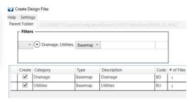
If existing drainage or utility graphics are contained with the projects Survey Fieldbook then the **Extract From Graphic** tool can be used to create existing drainage or utility models.
