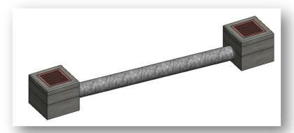
The link is placed at the lowest elevation of the selected nodes. The elevation values can be edited by selecting the link in either the 2D or the 3D model, and then choosing the **Properties** icon from the pop-up menu.
