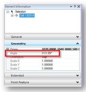
✓ Select the drainage node graphic and choose the **Properties** command from the pop-up menu. The **Rotation** can be modified as shown below. The graphics for the node in the 3D model are updated as changes are made to the properties.
