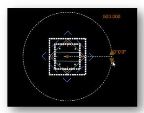
Selecting the graphic reveals a pop-up menu that can be used to make edits to the drainage structure as well as two rules (Node Top Elevation, and Node Rotation) that can be edited by selecting the displayed text.
