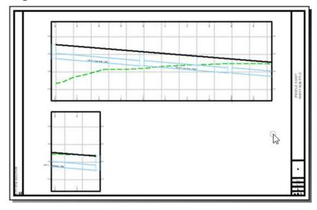
**Tip:** You can bulk create profile sheets for all profile runs by adding them to a selection set before starting the Place Named Boundary tool. There is a Graphical filter named Profile Runs which can be used with the **Select by Graphical Filter** Tool to help create the selection set.
