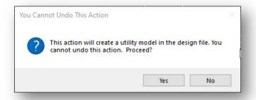
After the utility model has been created, the user must reselect the Drainage & Utility command to initiate the command.
