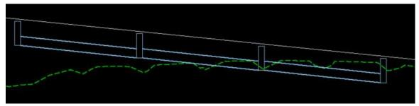
The profile run is projected perpendicular onto the alignment's profile. Notice if you turn off the DR\_P\_Storm\_Sewer level you will see the Profile run element on the SC\_ProfileRun1 level.
