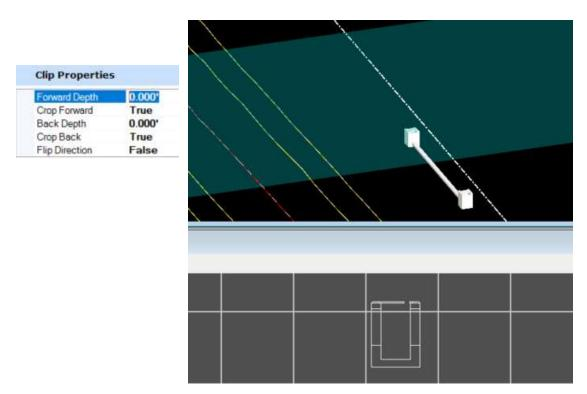
• After the value is updated notice how the connecting pipe shows up in the cross-section view. Now the connection pipe annotation can be added to the node. (Follow the steps outlined in the <a href="Profile View Drainage Annotation - Node Annotation Section">Profile View Drainage Annotation - Node Annotation Section</a>).
