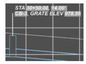
As mentioned above node annotation should be auto annotated during sheet creation. The **Model annotation** and **Element annotation** tools could be used as well. But the annotation is missing the information about the connecting pipes. Currently this cannot be auto annotated. Follow the below steps to add in the annotation for each pipe that connects to the node.
