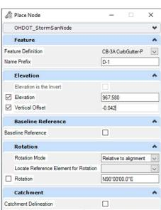
**Tip**: When entering a vertical offset value don't forget the negative sign to offset below the selected element. Also, basic calculations are supported for example to vertically offset 0.5" below the reference element you can enter -0.5/12.
