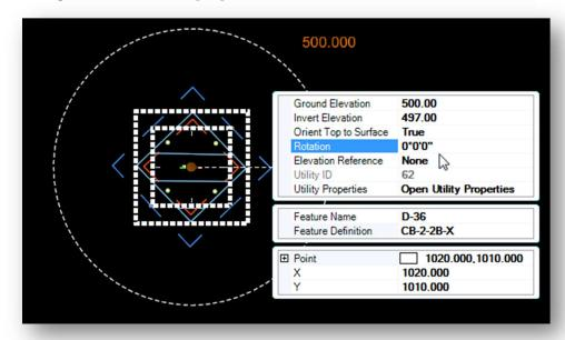
After extracting the drainage structures and rotating them into place we are ready to extract the pipes.
