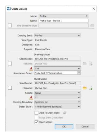
This will create a drawing model for each named boundary and sheet models. Annotation is placed in the drawing model.
