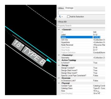
\*\* While annotation should typically be placed within drawing models. There are currently some bugs in the software, and it is best to place these pipe annotations in the Drainage Basemap file. \*\*
