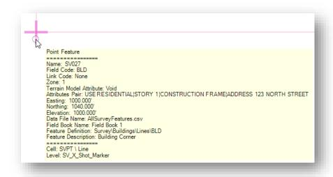
If the building is annotated, using the **Annotate Element** command, the text is constructed from the attribute data and placed on the level **BD\_X\_Text** like the example below.
