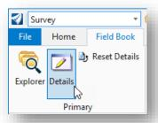
The content of the dialog is determined by the selected item in the *Explorer* dialog's *Survey* tab. In the example below, the Survey points that have the CMON feature definition assigned are displayed.
