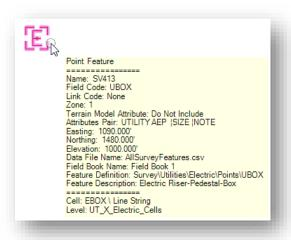
The **Element Selection** command can be used to review or edit various properties of a selected point. When a point is selected, a menu of commands will appear onscreen as shown below.
