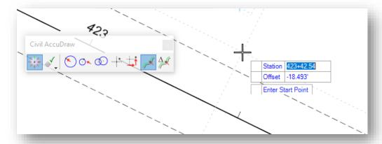
The reference element can be a MicroStation element or an ORD Geometry element. If a MicroStation element is selected, the beginning of the element is assumed to be station 0+00. If a civil element is selected with stationing defined, the station value of the selected element is used.
