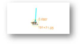
Notice the stationing is not visible upon completion but is ruled to the geometry. To check, select the element and look at the beginning to see the station. This is one place the stationing can be adjusted as well.
