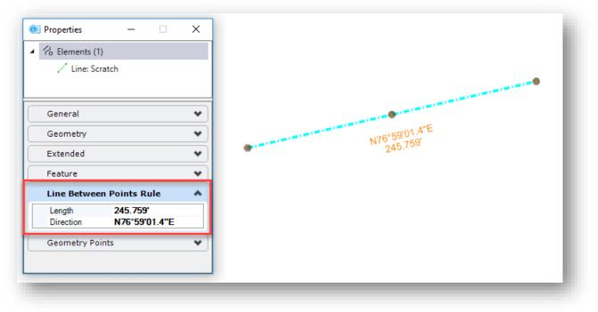
MicroStation's **Manipulate** commands (Copy, Move, Scale, Rotate, etc.) cannot be used on ruled geometry. The rule must be removed to use these commands. To remove a rule, select the line and choose the Rules menu as shown below.
