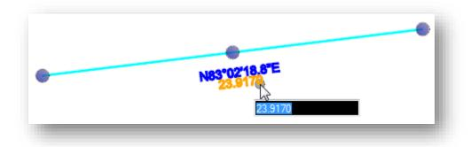
Clicking on one of the key point manipulators will display direction arrows to edit the line, as shown on the example below.
