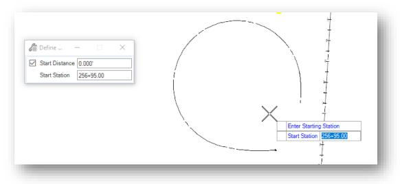
Annotate the alignment using the Survey > Drawing Production > Annotations > Element Annotation command. The stationing and curve data are annotated like the example below.
