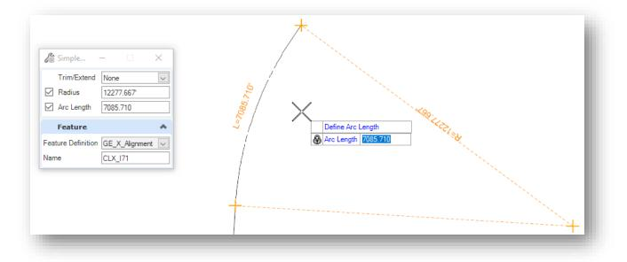
At this point, two separate pieces of geometry have been created. These elements can now be combined into a single alignment using the **Complex Geometry** command.
