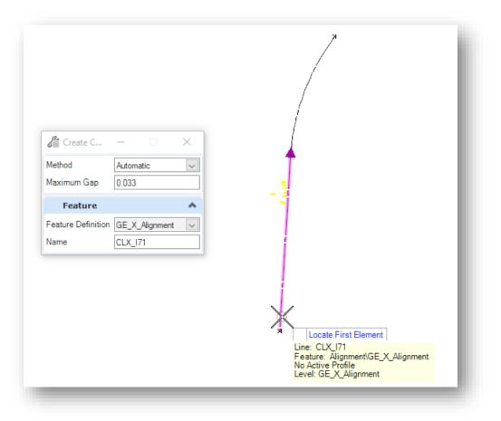
The elements are joined together as a single complex element.
