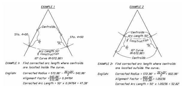
The diagram of the example showing the method of correction should be shown on the General Note Sheet. The corrected arc lengths should be shown in the earthwork tabulations on the cross-section sheets.
