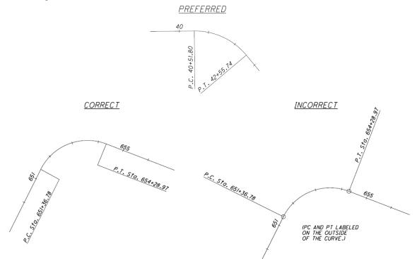
When space prohibits or when an alignment has a large number of horizontal curves, label each curve and tabulate the curve data. If it is necessary to tabulate curve data for a few curves along an alignment, then all curves should be tabulated to provide consistency.
