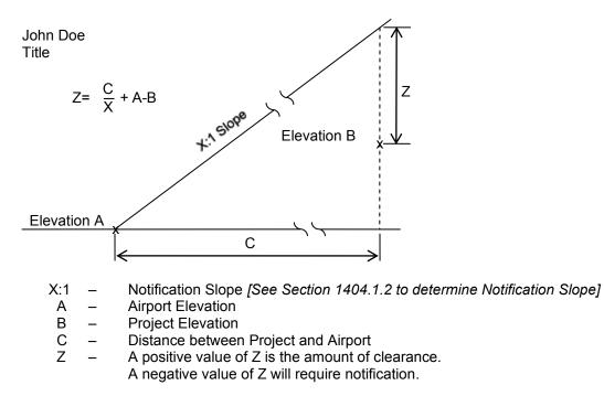
[The Z value should be calculated at critical points for projects of considerable length and variable heights (i.e. closest point, highest point, etc.).]
