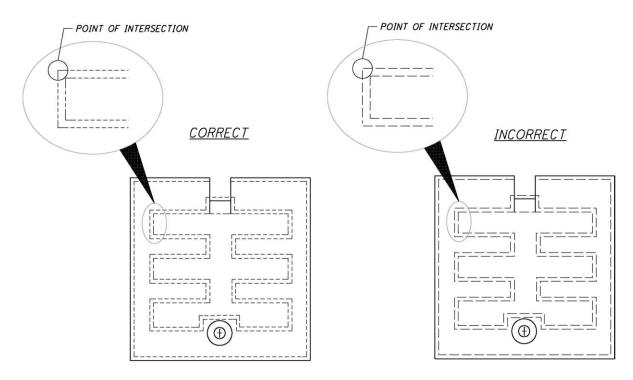
When needed for clarity, a gap should be shown at all locations where a visible edge becomes hidden by another surface as shown below.
