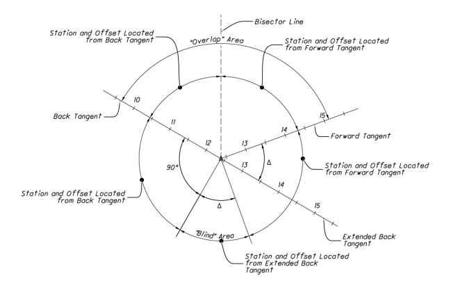
In addition to the "overlap" area, there is a "blind" area in which a station and offset cannot be measured from either the back or forward tangent. Stations and offsets in the "blind" area should be measured off an extended back tangent as shown in the figure.
